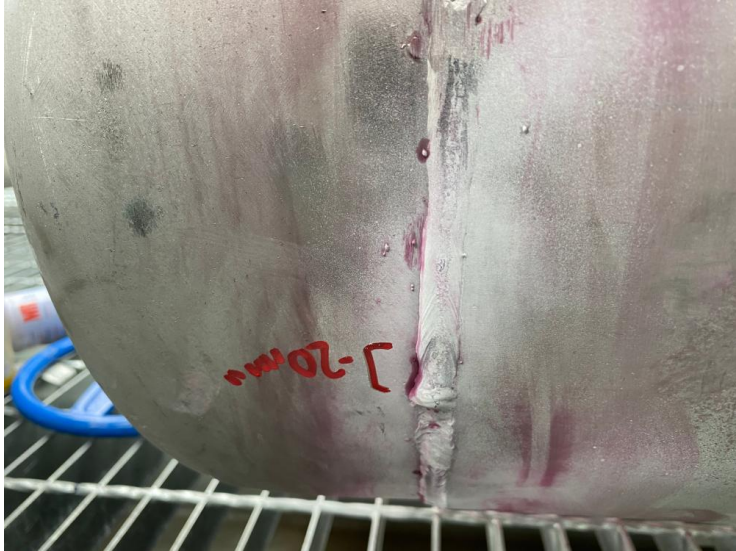
Image 13 of 13 - Spool 2 W6- 20mm overlap/ lack of fusion
