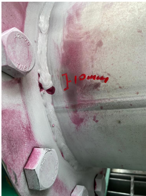
Image 8 of 13 - Spool 2 W3- 10mm overlap & poor stop/start
