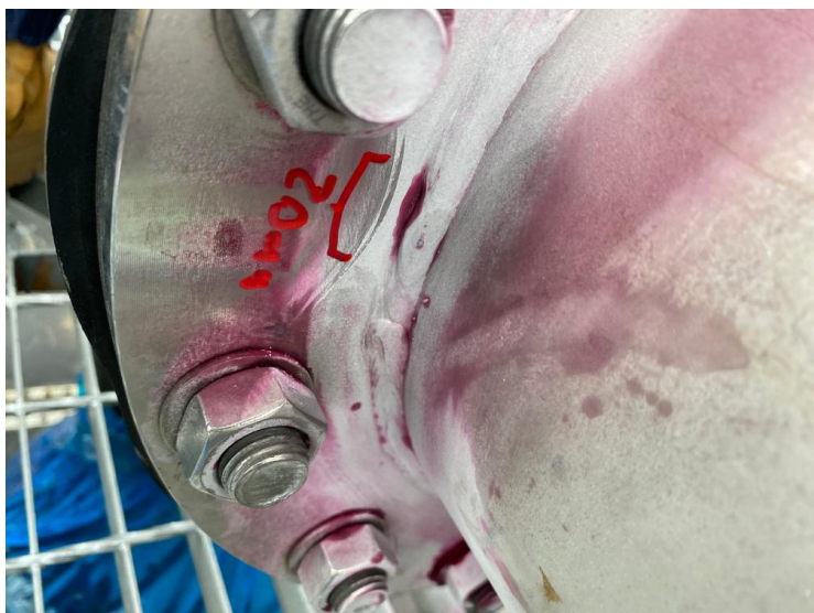
Image 11 of 13 - Spool 2 W5- 20mm overlap/ lack of fusion
