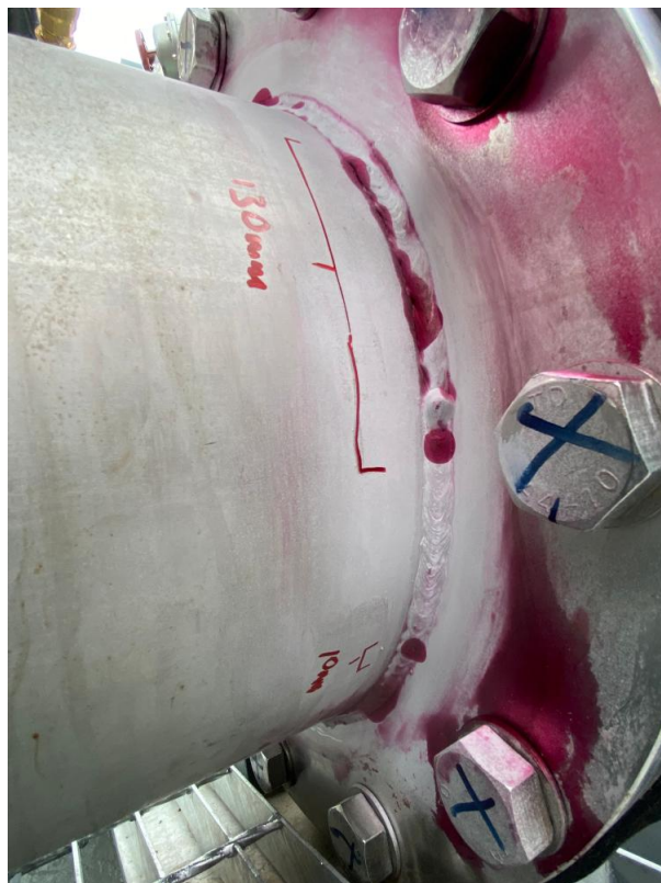
Image 4 of 13 - Spool 2 W1- 130mm overlap/ lack of fusion; 10mm porosity
