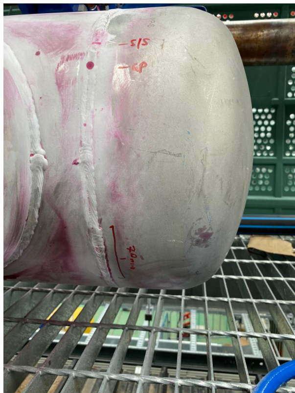
Image 12 of 13 - Spool 2 W6- 70mm overlap/ lack of fusion; 10mm poor restart; 10mm porosity
