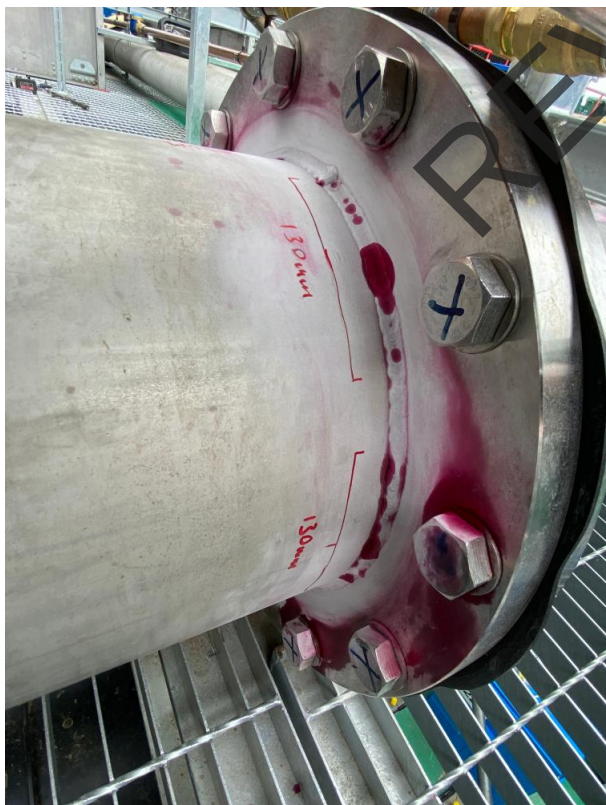
Image 3 of 13 - Spool 2 W1- 130mm linear porosity
