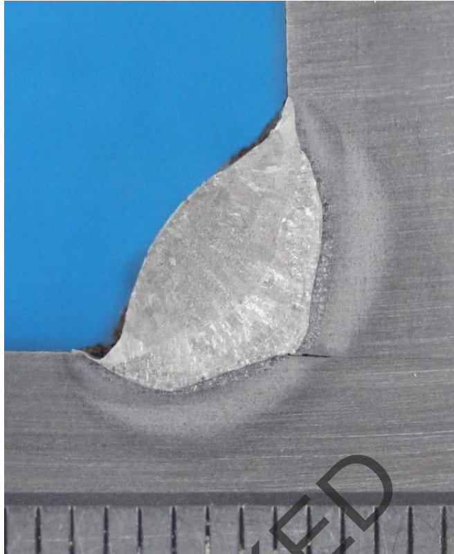
Image 1 of 2 - Macro Specimen 1 (1 Graduation = 1mm) M1
